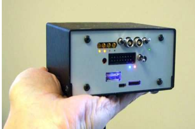
Figure 1: The FemtoDAQ provides two ADC channels (coaxial connectors in the middle) and a logic bus with detector bias supply (rectangular connector below analog inputs).
